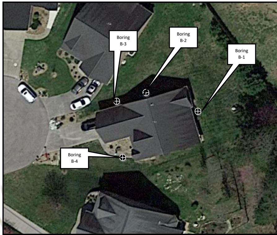
Figure 4: SPT Boring Location Map
